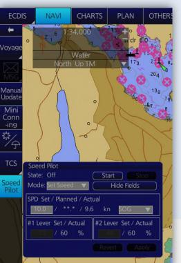
**Set Speed mode** allows for direct control of the vessel's speed by specifying desired speed. It is particularly useful when a speed needs to be maintained consistently.
